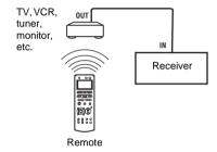
The remote sensor on the CTRL S OUT component receives remote codes the same way as the remote sensor on this unit. This is useful if you have placed this unit in a rack, etc.
